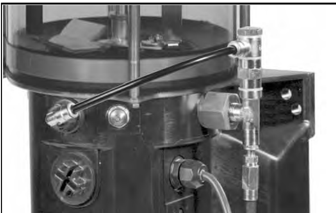
Fig. 5-2 Pressure relief valve with grease return
